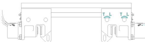
5' Caisson Beam with Model 100BH Caisson Clamps Clamping force 220 tons, 1975 kN Weight 3,000 lbs, 1360 kg
